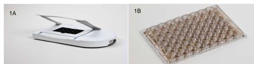
Figure 1A. The Maestro, Axion BioSystems. 768 recording channels with fully integrated heater and software controls. Accommodates 12, 48 and 96 well MEA plates. Figure 1B. 48 well configured MEA plate, Axion BioSystems. 16 microelectrodes per well, ANSI compliant, nano-textured gold electrodes with evaporation reducing lid.
